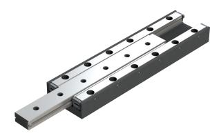
Frictionless low profile slides model RTS are fine preloaded linear motion units, ready for mounting. This low profile type offers an excellent running motion accuracy and is able to carry medium loads and moments in every direction.
